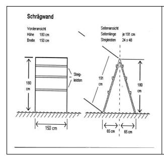
The scaling wall consists of 2 sides joined at the top and must be 150 cm wide and 190cm high. At the bottom both sides stand apart so that there is a peak height of 180cm The entire area of the scaling wall must be covered with anti skid material. At the upper part of the sides 3 cleats 24/48mm must be fixed. All dogs must jump the same obstacles.
